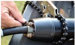
**EASIER TOOL MAINTENANCE.** Tailbolt system provides easy access for tool maintenance, requiring a maximum of only 35 ft-lb (47.5 Nm) of torque.
